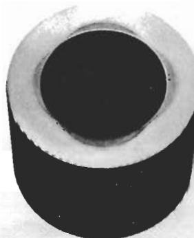
VASCOMAX C-350 Cold forming die for plow bolt heads. Best previous die material was D-2 — yielding an average of 3000 pieces. VascoMax gave 8000 pieces before cracking occurred.
