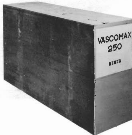
VASCOMAX C-250 Huge (16" x 30" x 55") high quality forging as furnished by Teledyne Vasco for a die casting customer.
